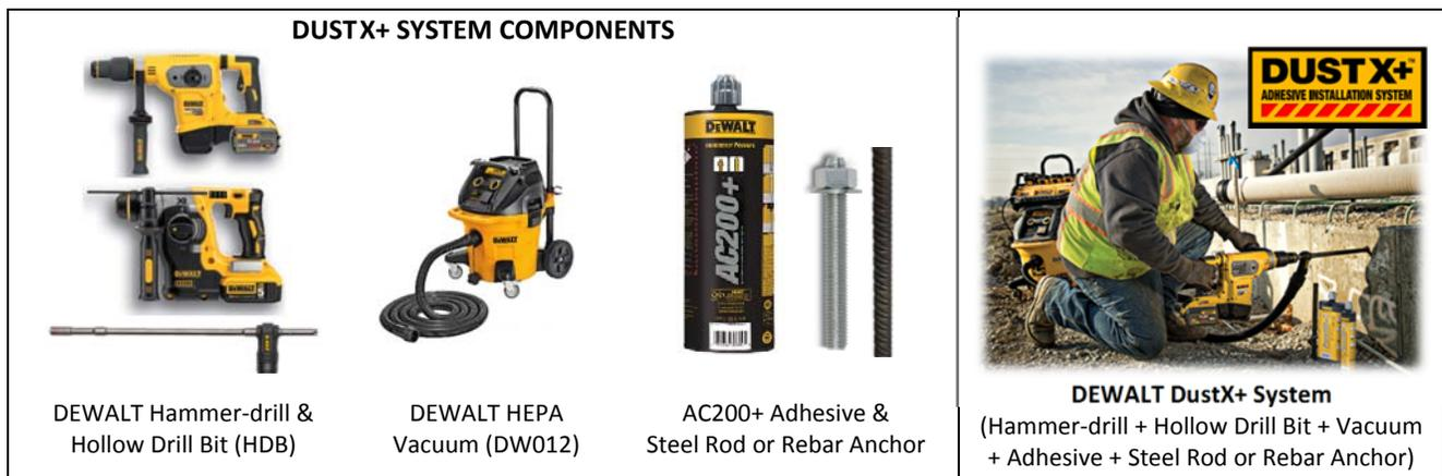
The DustX+ system allows users to drill holes in concrete and clean the holes during the drilling process at the same time (no extra cleaning steps are necessary with this system). The hollow drill bits are attached to a self-cleaning HEPA vacuum which provide the dust collection during drilling. DEWALT has conducted extensive supplemental laboratory testing on AC200+ adhesive anchors installed in holes drilled and cleaned using the DustX+ system in dry concrete.
